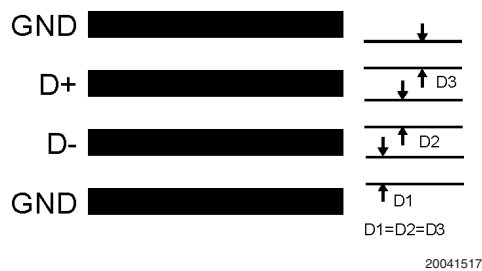
FIGURE 11. Ideal Diode Trace Layout
